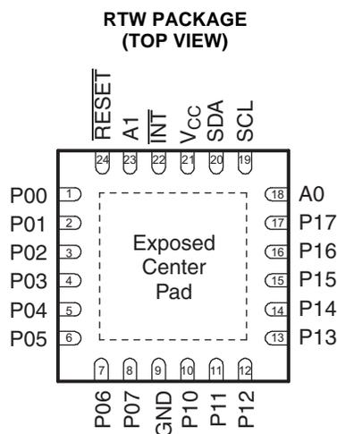
The exposed center pad, if used, must be connected as a secondary ground or left electrically open.
